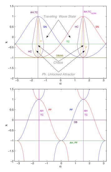
FIG. 8. (Color online) Bifurcation diagrams on the  $(\alpha,k)$  bifurcation plane for four oscillators: (top)  $N_1 = 3, N_2 = 1$ ; (bottom)  $N_1 = N_2 = 2$ . Notation: AH, Andronov-Hopf; SN, saddle node; PF, pitchfork; TC, transcritical; F, fold of cycles; HC, homoclinic; DB, degenerate bifurcations.
