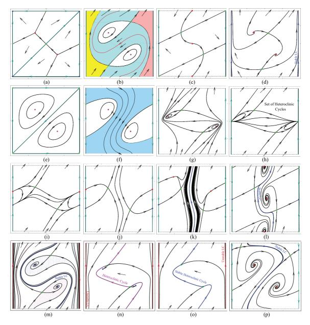
FIG. 6. (Color) Phase portraits for  $\phi_1, \phi_2 \in [0, 2\pi)$  for two conformists and one contrarian. The cases a, b,..., p of the bifurcation diagram of Fig. 5 (top) are represented for different values of the parameters  $\alpha$  and k. Point types: red, source; blue, sink; green, saddle; magenta, center; dark green, saddle node. Stable limit cycles are shown by blue; unstable limit cycles by red. Two-dimensional color regions indicate the sets of nonisolated periodic orbits.
