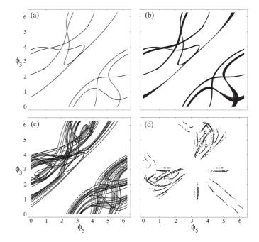
FIG. 3. Projections on the plane  $(\phi_3, \phi_5)$  of some trajectories of system (5) for  $N_1 = N_2 = 3$ : (a) periodic trajectory (k = -0.21), (b) quasiperiodic trajectory (k = -0.216), (c) chaotic trajectory (k = -0.3), (d) Poincaré section  $\phi_4 = \pi$  (k = -0.3).
